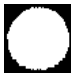
Figure 1: Approximate circular structuring element, radius 25, constructed using 8 lines.
