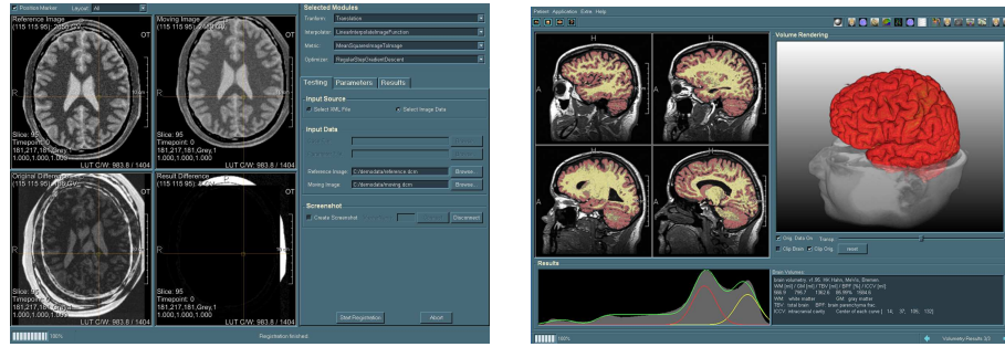
Fig. 3. Combining ITK and MeVisLab for the generation of flexible test environments and rapid application prototyping. (LEFT) Test environment for evaluation of ITK image registration algorithms. The data were obtained from the BrainWeb project [13]. (RIGHT) Application prototype for semi-automatic brain volume quantification used for diagnosis support and therapy monitoring.
